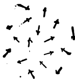
FIG. 10.—HETEROGENEOUS ASSOCIATION, CORRESPONDING TO ABSENCE OF MAGNETIZATION.
